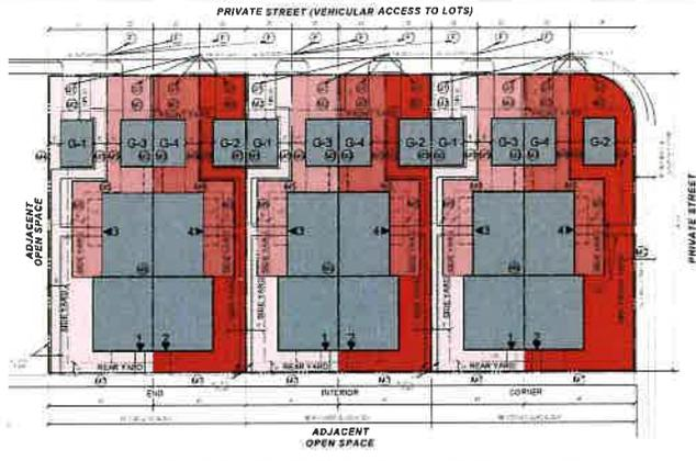
SPEX DETAIL: QUADRUPLEX TYPICAL LOT LAYOUT (ADJACENT OPEN SPACE AT REAR)
